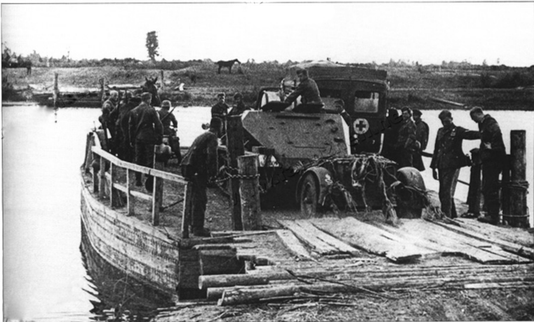
A Sd.Kfz. 252 from a battery of self-propelled howitzers (probably a sIG 33 battery) crosses a river in the Smolensk area in September 1941. The Sd.Kfz. 252 was a half-track armored ammunition carrier built in the same manner as the Sd.Kfz. 250 armored personnel carrier.
