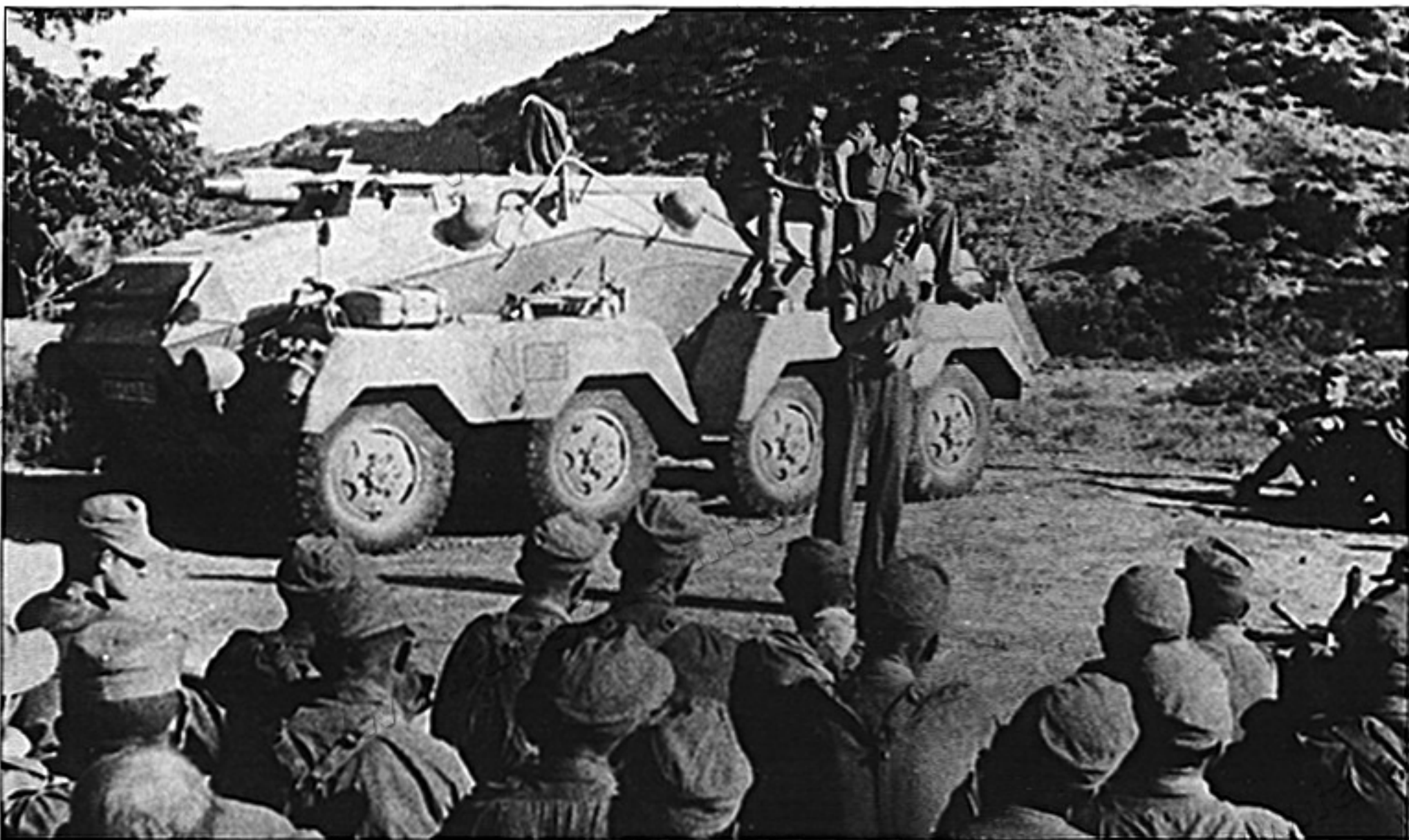
Another shot of an armored recon unit on Rhodes, this time showing a Sd.Kfz. 233. This is an early model of this vehicle and can be easily distinguished from the later version by the lack of the raised superstructure around the combat compartment. The vehicle was designed in autumn 1942 to be a heavy support vehicle for reconnaissance troops.
