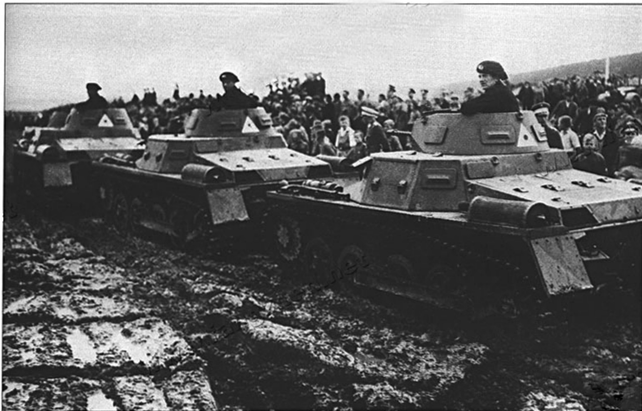
A platoon of four Pz.Kpfw. I Ausf. A negotiates some muddy terrain during a show for civilians. Note the pattern of camouflage partially visible on the two nearest tanks. Of special interest are the tactical markings composed of a white triangle with a black circle inside painted on the rear of the turrets. The Pz.Kpfw. I was a simple tank that suffered many problems due to its chassis, which prevented it from covering difficult terrain at combat speed during battle.
