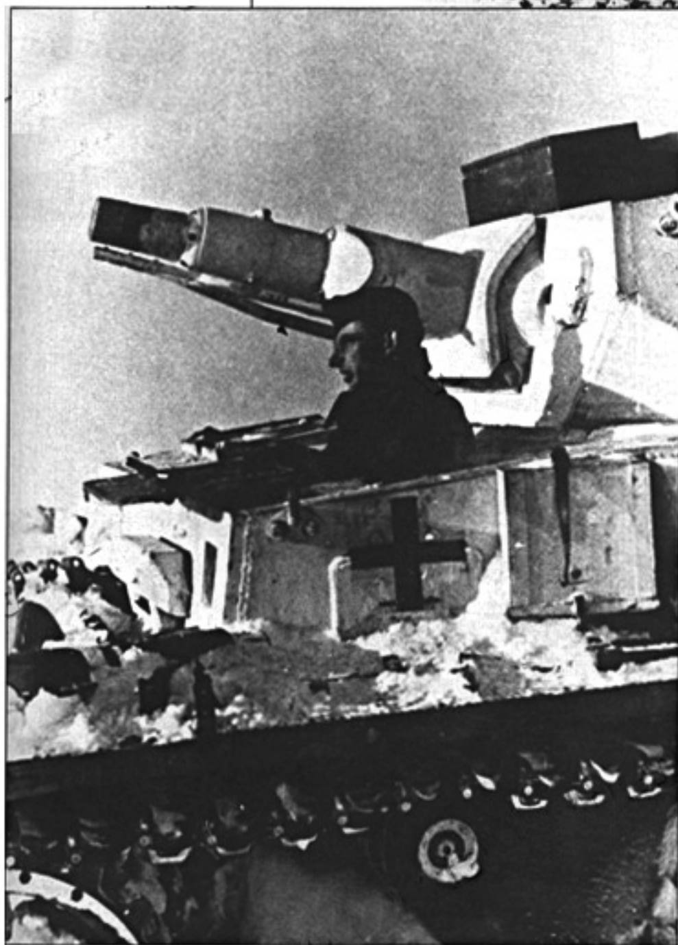
A close-up photo of a PzKpfw IV Ausf. E employed in 5. Panzer-Division during early 1942. A yellow division insignia painted on a dark gray background is visible near the edge of the front plate of the superstructure, where it is outlined with white camouflage paint. Below the driver is a national cross whose white outline is darker than the coat of white camouflage. This was typical because the white paint of markings absorbed dirt very quickly, transforming the white color into gray, cream, etc.
