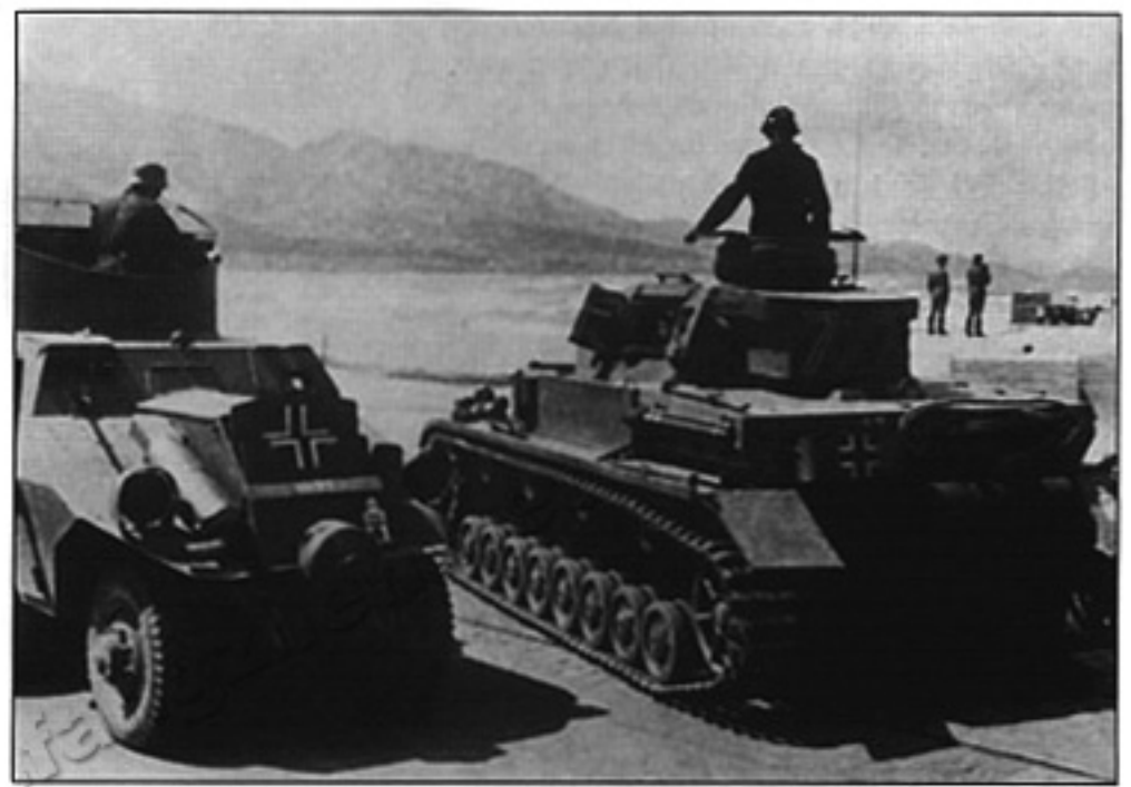
A Pz.Kpfw. IV Ausf. E or Ausf. F1 with a short-barreled gun passes by a heavy AGDZ armored car on a street near the Mediterranean coastline of southern France. Both vehicles carry the same unit markings — a white tower with a gate.
