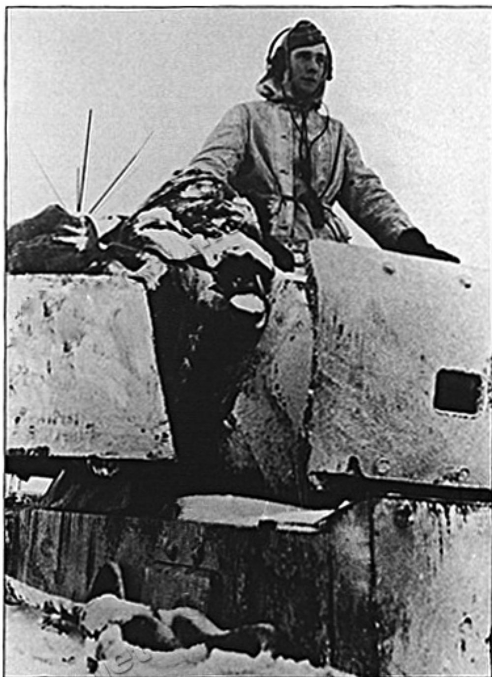
A warmly dressed tank commander keeps alert in the cupola of a Pz.Bef.Wg. III Ausf. K. This photo shows to advantage the details of how camouflage paint was applied. Visible behind the turret is the winch antenna mast of a FuG 8 radio set. This type of antenna, which was introduced in 1942, soon replaced the frame antenna. The FuG 8 was used to command tank troops, but some Pz.Bef.Wg. IIIs were equipped with the FuG 7 for communication with the Luftwaffe.
