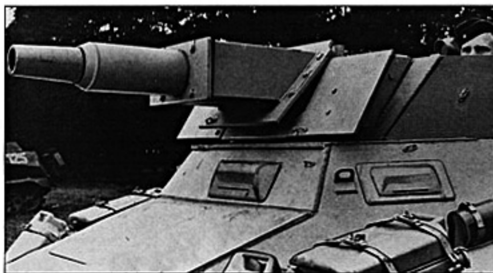
The Sd.Kfz. 234/3 was issued to armored reconnaissance companies to provide anti-tank support for other armored cars. Produced in the latter half of 1944, these vehicles mounted a 7.5cm L/24 howitzer. Note the details of the gun mount. In the background may be seen the rear portion of a Sd.Kfz. 250/9, the reconnaissance version of the Sd.Kfz. 250, which was armed with a 2cm gun installed in a turret taken from a Sd.Kfz. 222.
