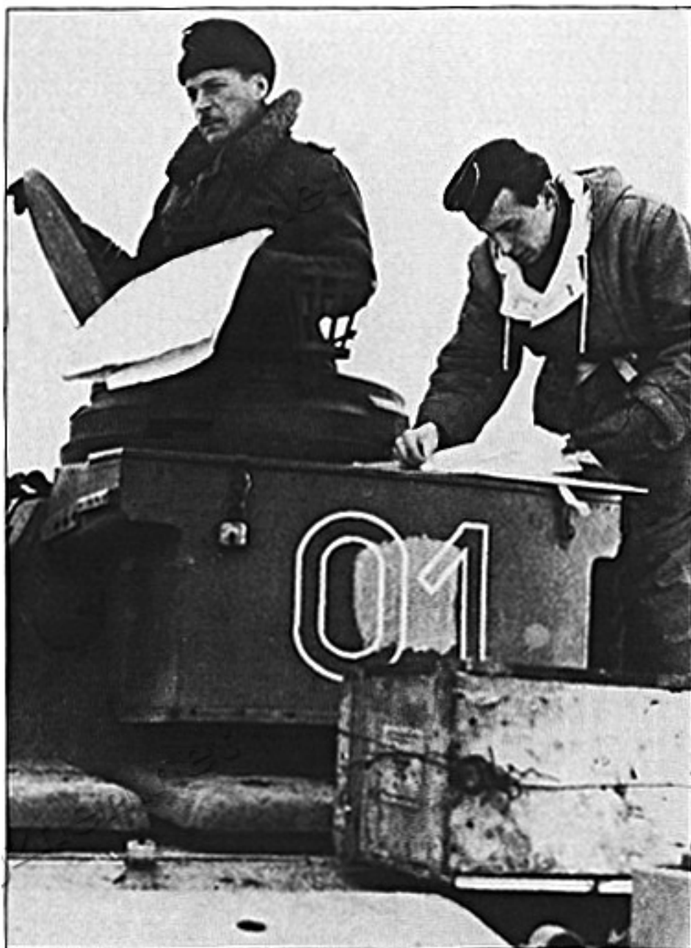
Oberst Graf Strachwitz, commander of Pz.Rgt. "Großdeutschland", consults a map during the fight for Kharkov in March 1943. He is seen here in the cupola of his Pz.Bef.Wg. III's turret, which is marked with the tactical number "01" on the stowage bin. Note the strange fixture attached to the cupola just below his left arm. Such items were often seen on the command versions of the Pz.Kpfw. III during this period. Graf Strachwitz often used command tanks because he spent a lot of time on the battlefield directly commanding his units.
