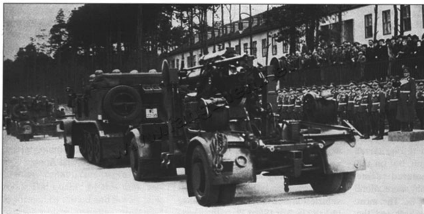
A similar view showing an early Sd.Kfz. 7 armed with a 8.8cm Flak 36 anti-aircraft gun, seen from the rear in this photo. Note the white letter "B" painted on the gun just below the barrel. The license plate of the prime mover reads "WL 221135".
