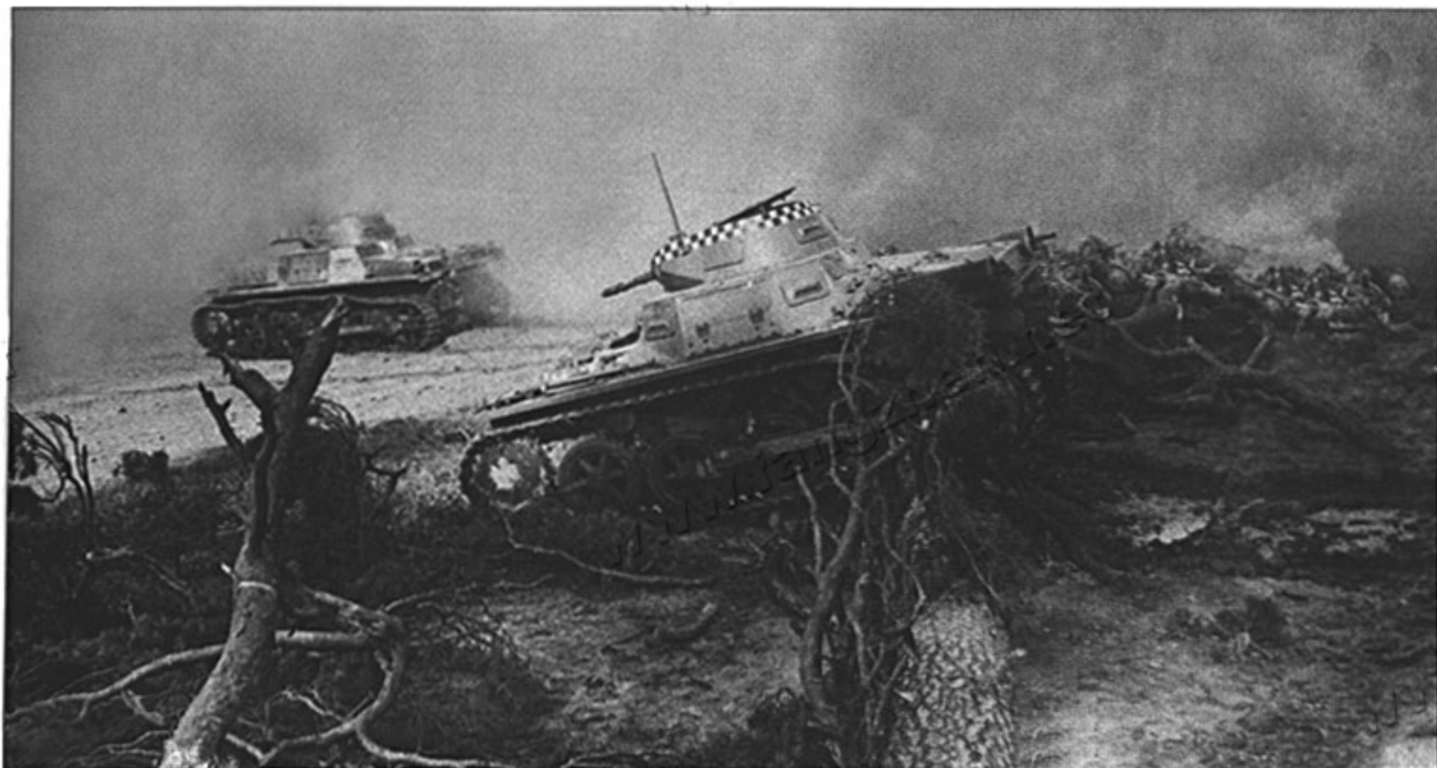
Two Pz.Kpfw. I Ausf. A maneuver during a training exercise. The Pz.Kpfw. I was quite fast and maneuverable, but its chassis and engine were too weak. Note the black and white checkerboard pattern on the top of the turret. The pattern, which has been painted around the turret, can also be seen on the mantlet. The Germans used this sort of marking to indicate the command tanks for a short period in the first half of the 1930s. Note that the tank in the background does not feature such markings. This fact would seem to dispel the theory held by some scholars of German armor that the checkerboard is an identification marking for "enemy" forces during field maneuvers, as it has been sometimes claimed. Note the illegible markings on the Pz.Kpfw. I in the background that have been painted just under the turret on the rear plate of the superstructure.
