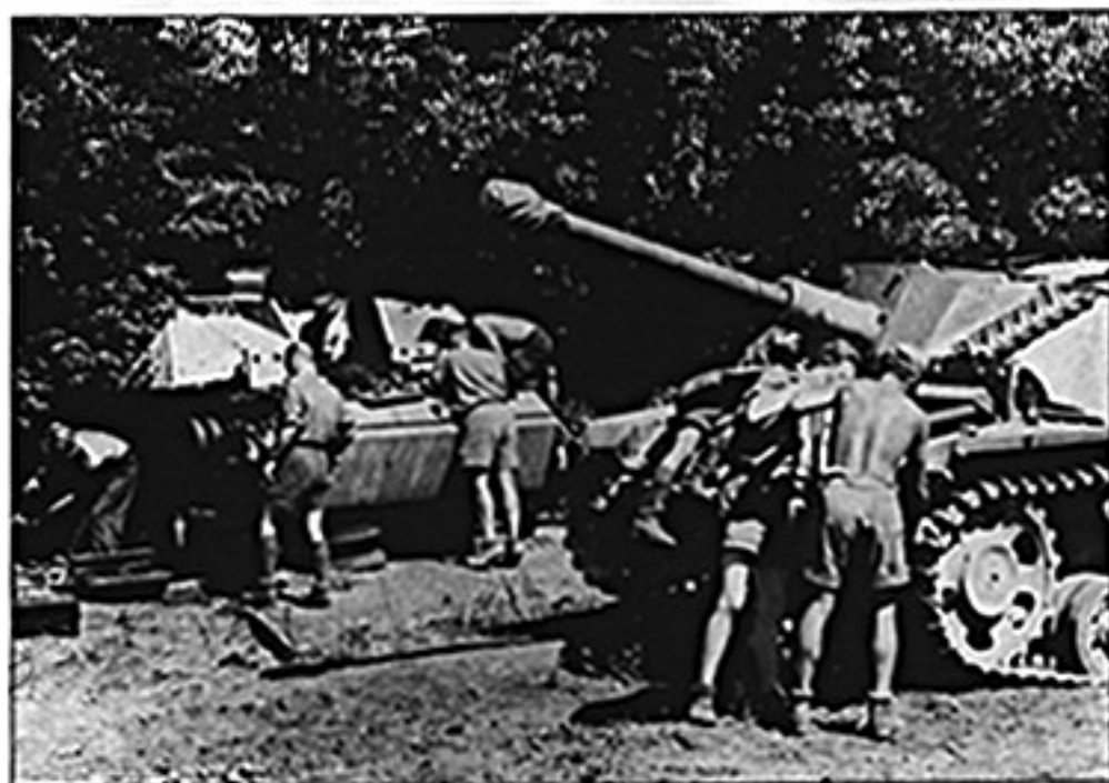
This photo shows a workshop concealed somewhere in the woods on the Western Front that was set up just prior to the Normandy invasion. The vehicle in the background undergoes a thorough repair. Both the sprocket and final drives, and the complete gun assembly, have been removed. The other vehicle apparently has problem with its brakes.
