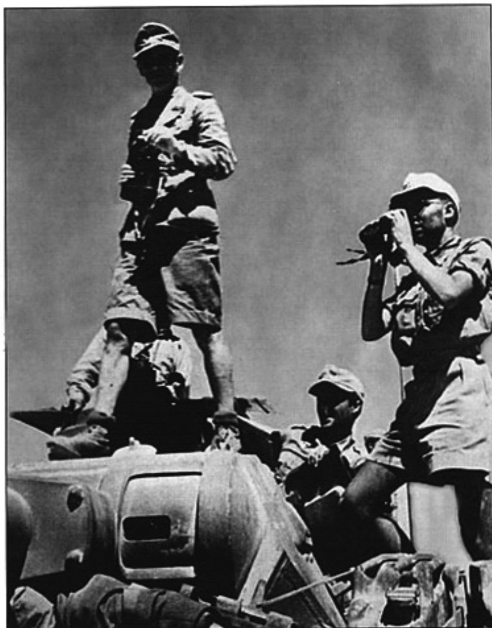
General Erwin Rommel, seen here with General Georg von Bismarck, directs a battle from the combat compartment of a Sd.Kfz. 251/6, probably von Bismarck's vehicle. The "Hanomag" still has the remains of its original dark gray camouflage in places where the new coat of sand paint was not applied. Due to a lack of equipment and water, the sand paint was usually applied as a paste with brushes, as is visible in this photo. The three-color lance pennon (from top to bottom: black, white and red) above the machine gun shield indicates the staff of 21.Panzer-Division.
