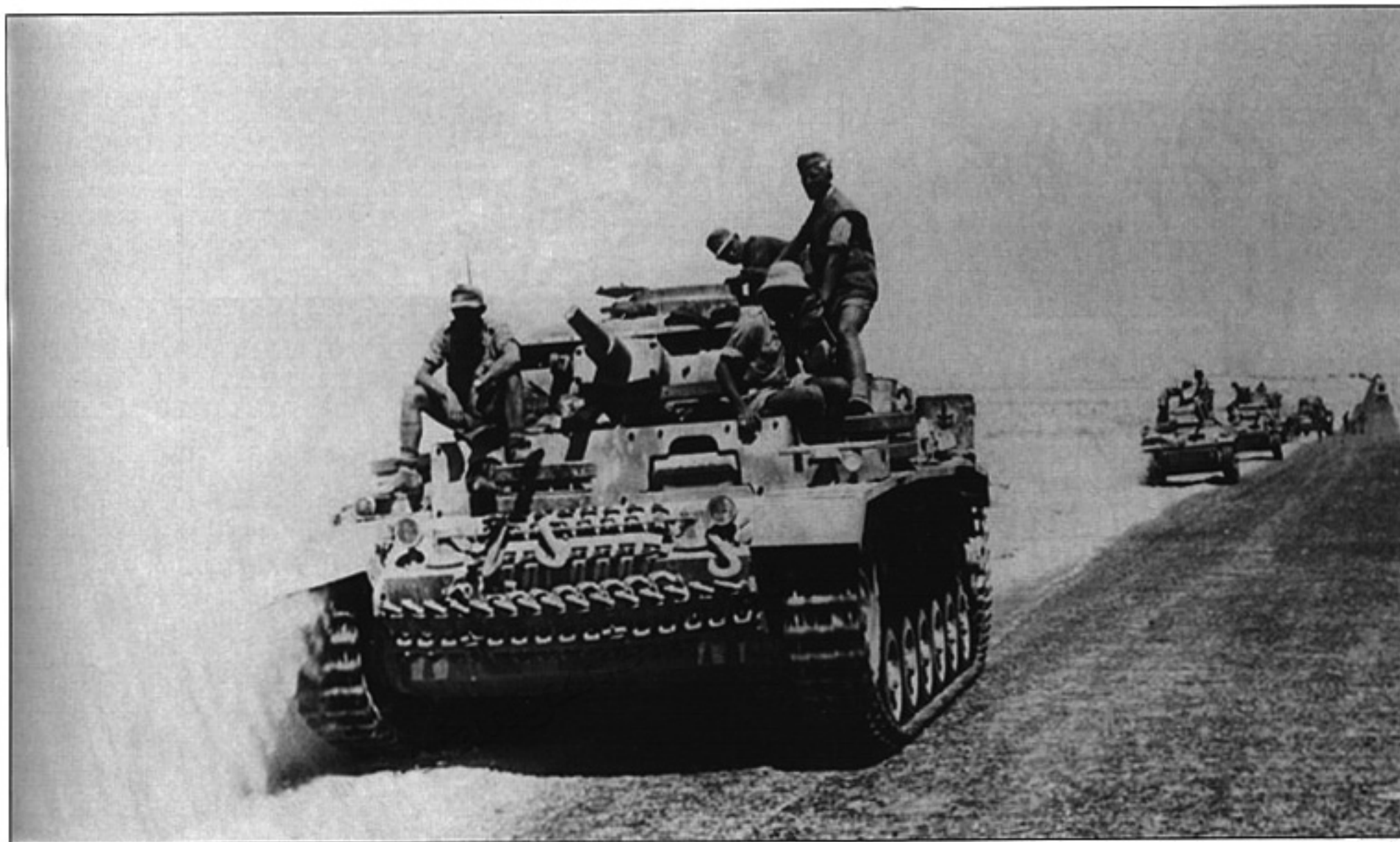
The newest model of the Pz.Kpfw. III, the Ausf. J, arrived in Africa in the summer of 1942. It was armed with the old short-barreled 5cm gun, but with new additional armor plates. One of these tanks is seen here en route to the front line deep inside Egypt in July 1942. Note the pattern of colors on the front plate of the superstructure, which looks like camouflage composed of two different paints: sand (RAL 8000) and green-gray (RAL 7008). Such paint schemes were very rarely seen on DAK vehicles. The two-tone camouflaged armored fighting vehicles are usually seen in photos taken in the middle of 1942. During Operation "Venezia" the DAK suffered the loss of 175 Pz.Kpfw. IIIs out of a total of 233 destroyed tanks. But at the same time, German tank crews claimed 790 enemy tanks and 170 other armored fighting vehicles.
