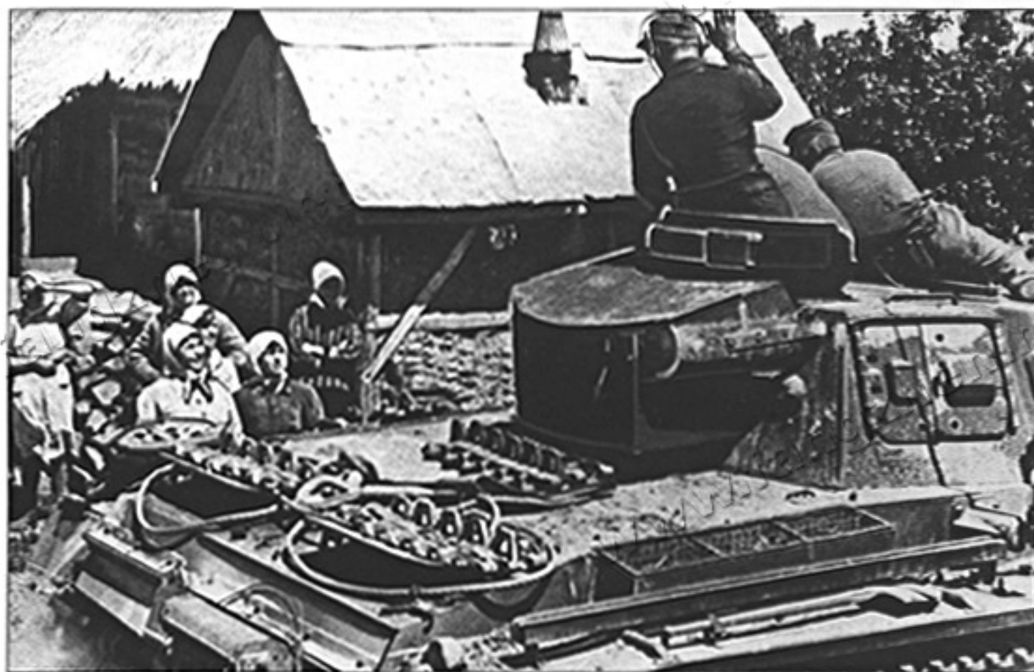
Panzer crewmen of a 7th Panzer company extend greetings to some Ukrainian peasants in July 1941, a time when many people on both sides thought that there could be friendly relationships between them. Based on the details visible on the engine deck of the tank seen in the photo, it appears to be one of the 600 Pz.Kpfw. III Ausf. Gs produced up to February 1941. Like most German tanks of this period, this Pz.Kpfw. III is fitted with smoke candle dischargers.
